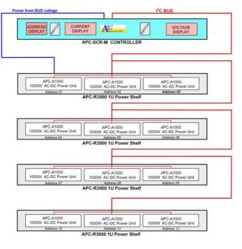
Up to 12 hot swap power units can be used in parallel and the controller can be used to select a particular power unit position and read the current being drawn from that unit with a resolution of 100 mA. The address of individual power cartridge is set in hardware using the cable assembly supplied with the controller.
