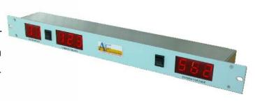
The controller is digital and communicates with the power modules by means of an I<sup>2</sup>C bus.
