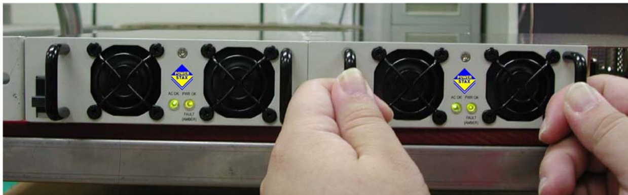
Step 3 : Push fully home and PWR OK LED is ON.
