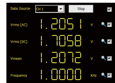
Measure 1 KHz, 2.5 Vpp square waveforms by the DVM function.
