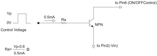
Note: The control voltage is referenced to negative input (-Vin)
