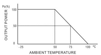
Note: At nominal input, Full load and cooling is natural convection.
