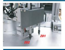
High reliable pick-place  ${\bf Z}$  axis combines with high-precision firm-nozzle.
